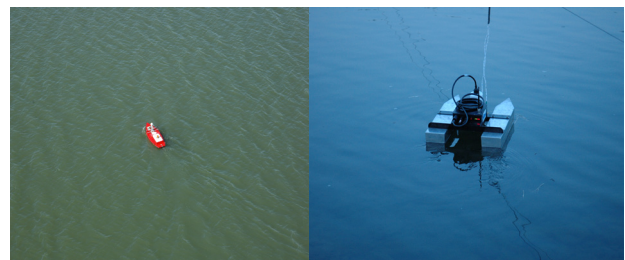
Fig. 4-5 Remote control boat and ADCP
